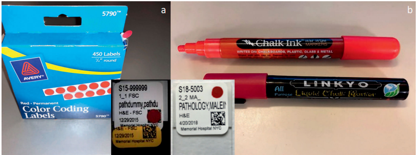
Figure 4. Glass slide scanning indicator: composite red dot stickers with chalk ink. a, Color-coding label stickers; inset: sticker shown covering outside hospital barcode. b, Liquid chalk ink markers; inset: chalk ink dot shown in upper right hand corner of slide label as slide scanning indicator.
